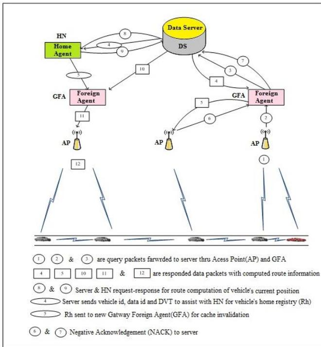
Fig-3 Architectural Proposal along with Service Mechanism
