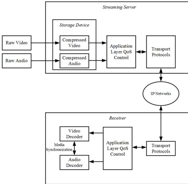
Figure 1: A typical video streaming architecture
