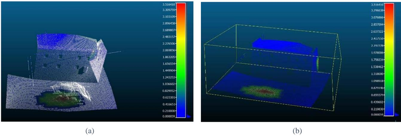
Figure 5.output point cloud presented in gradient colours, different colour shades represent the directional changes between the different point clouds acquired at different times; ; Reddish and greenish shades dots signify possibly change events, while bluish represent stable actions within resolution cell accuracy (a) the proposed method. (b) Clustering algorithm.
