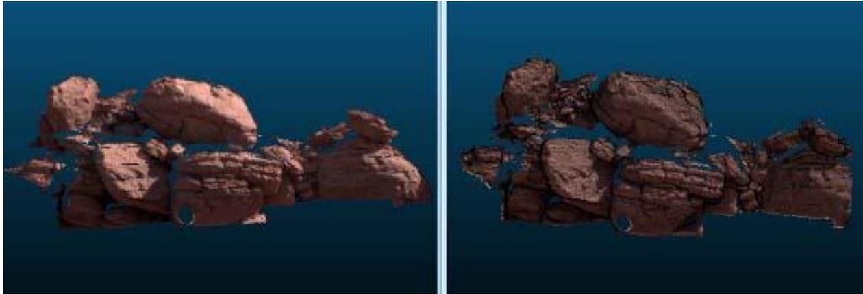
Figure 3. Example real LiDar scan data from the optech ILRIS acquired at different time, this reepresents an extracted section of the original data; due to the scanner position the angular nature affect the rock positions
