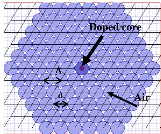
Fig.1 structural parameters of PCF
