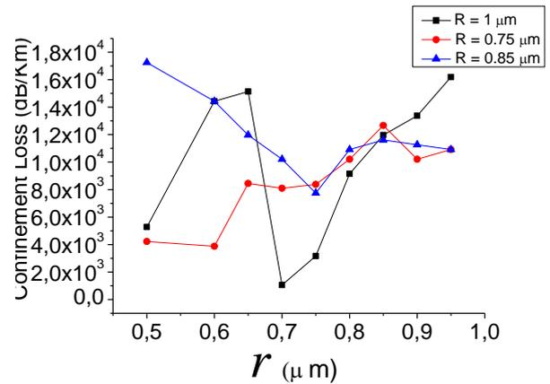
Fig.9 Variation of confinement loss with the variation of the minor radius  $r$
