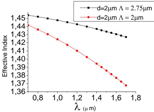
Fig.2 variation of effective index with the wavelength
