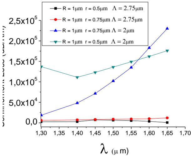
Fig.7 Variation of confinement loss with the wavelength case of PCF with elliptical air holes
