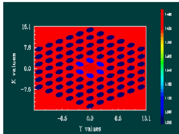
Fig.10 The distribution of the refractive index
