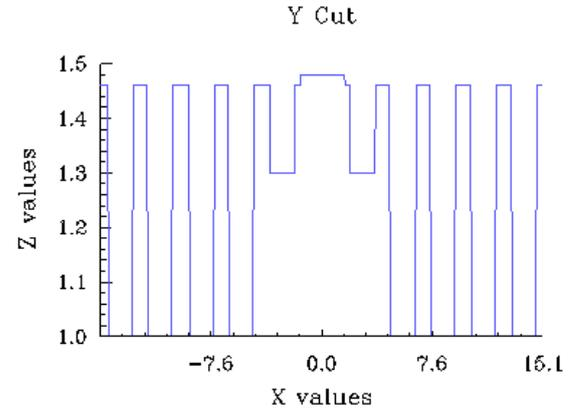
Fig.12. Profile of the refractive index of the structure (Y cut) for  $n_L=1.3$
