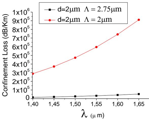
Fig.3 Variation of confinement loss with the wavelength
