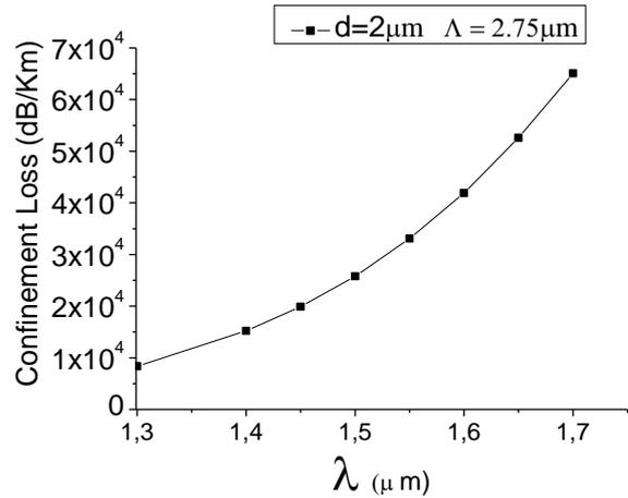
Fig.4 Variation of confinement loss with the wavelength case of  $d=2\mu\text{m}$  and  $\Lambda=2.75\mu\text{m}$
