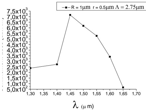
Fig.8 Variation of confinement loss with the wavelength case of  $R = 1\mu\text{m}$   $r = 0.5\mu\text{m}$   $\Lambda = 2.75\mu\text{m}$
