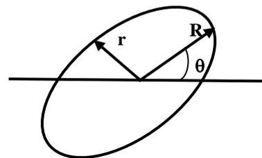
Fig.6. minor radius  $r$ , Major radius  $R$ , and orientation angle  $\theta$
