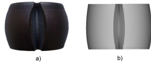
Figure 2. Shape of deformed test sample at temperature 700 °C a) laboratory experiment b) computer simulation
