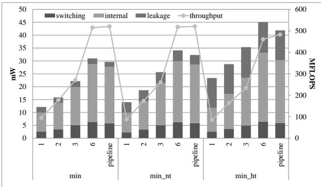
Figure 4. Average power analysis for scaling pipeline depth leakage power of the “min\_ht” library is higher than those of the others due to high temperature characteristics. Third, the power of the scaled six-stage pipeline is approximately 10% higher than that of the pipeline structure.
