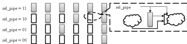
Figure 2. Pipeline control for a scalable 6-stage pipeline
