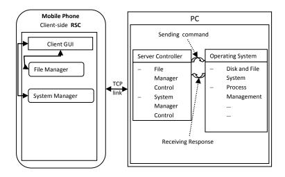
Figure 1: Basic Architecture of RSC
