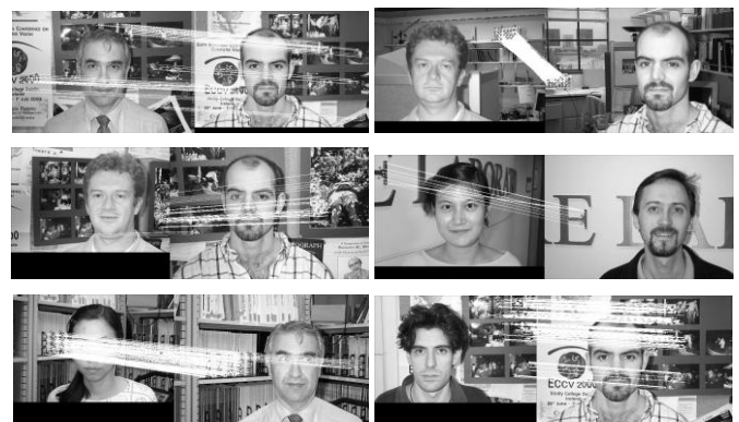
Figure 4. Examples of correctly retrieved similarly looking background fragments (even though the images contain different faces).
