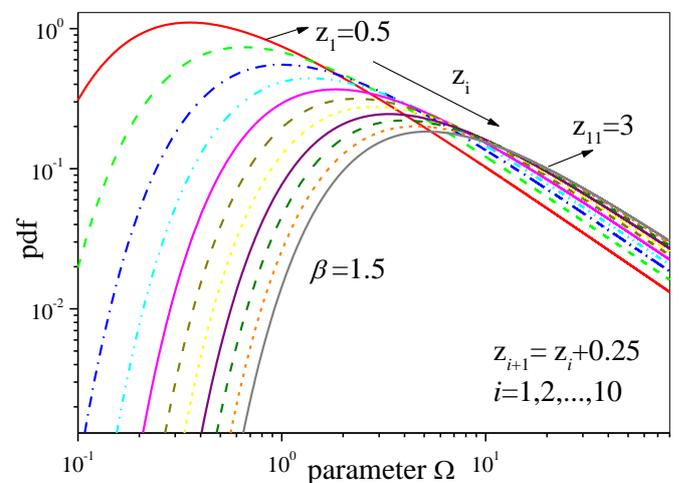
Figure 4. Weibull pdf versus  $\Omega$  for different values of  $z$  and  $\beta=1.5$
