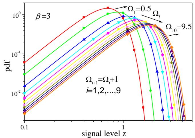
Figure 1. Weibull pdf versus  $z$  for different values of  $\Omega$  and  $\beta=3$
