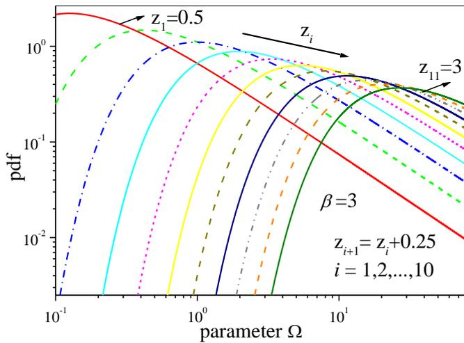
Figure 2. Weibull pdf versus  $\Omega$  for different values of  $z$  and  $\beta=3$
