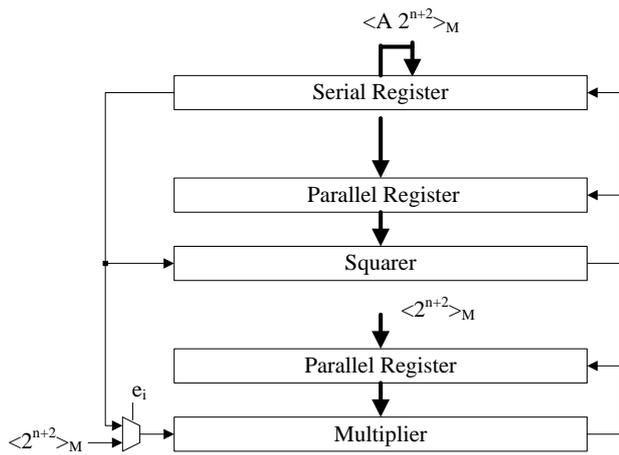
Figure 1. A Speed-Efficient (SE) RSA Structure that uses two multipliers
