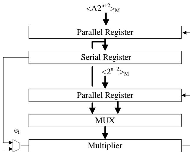
Figure 2. An Area Efficient (AE) RSA Structure that uses one Montgomery Multiplier
