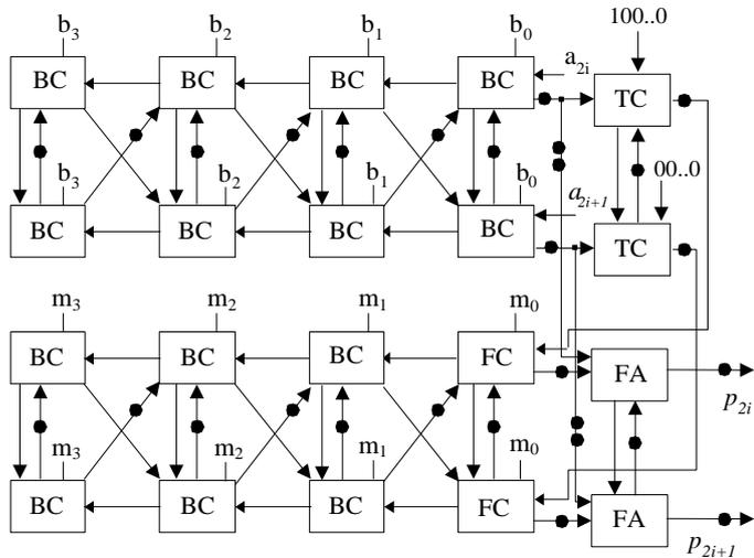
Figure 4. A 2-bit Digit Montgomery Multiplier that Implements Algorithm 3
