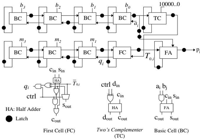
Figure 3. A serial Montgomery Multiplier derived from Algorithm 3
