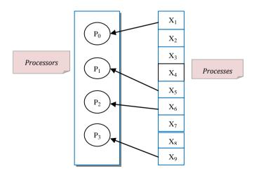
Figure-1: Multiprocessor system with maximum CPU utilization.
