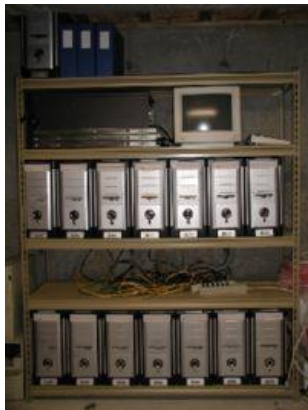
Fig. 2. A home-built Beowulf cluster [25]
