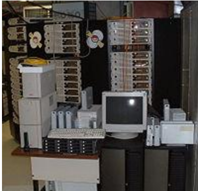
Fig. 1. A 52-node Beowulf cluster [25]
